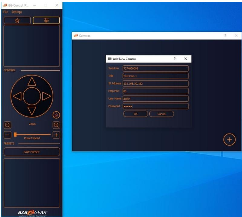
The serial number can be found on the box or a sticker on the base of your camera. Select **OK** when finished and your camera will be added to the application. Repeat the steps to add more cameras.
