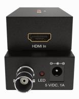
The BG-H3GS is a long-distance 1080P HDMI to SDI converter. This unit is designed to convert HDMI signals for use with SDI equipment. It supports resolutions up to 1080p60 at output distances up to 100 meters (3G-SDI), 200 meters (HD-SDI), or 300 meters (SD-SDI). This converter outputs high bit rates of 2.970 Gbps to provide a lossless high-resolution signal.
