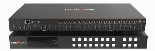
The BG-UHD-1616M is a 4K HDMI matrix switcher which supports video and audio from up to 16 sources to up to 16 HDMI displays. With this matrix, users can switch which display uses which input, enabling a great deal of control over many displays at once.
