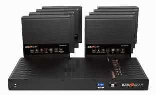
The BG-UDAIC-E14 and BG-UDAIC-E18 are HDMI extender and splitter kits that distribute one HDMI input to up to four (BG-UDAIC-E14) or up to eight (BG-UDAIC-E18) extender outputs.
