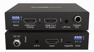
The BG-UHD-SC1X2 is a 4K 18Gbps HDMI Splitter with built-in Scaler, specifically designed for installations requiring a single 4K video source to be distributed to multiple displays that have video resolution limits. The BG-UHD-SC1X2 supports down-scaling of 4K video to a fixed resolution of 1080p or to a lower color gamut if the screen does not support 4K (4:4:4) using the HDMI Scaler Port. It also offers audio Embedding and De-embedding, advanced EDID management and is HDCP 2.2 compliant.
