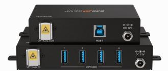
The BZBGEAR BG-EXUF is a 4-port fiber optic USB 3.1/2.0/1.1 extender that extends USB 3.1 up to 328ft (100m) and USB 2.0/1.1 up to 6.2mi (10Km) over single-mode or multi-mode fiber optic cabling. Designed with a four-port hub to extend up to four USB devices without the need for an additional device. Each port supports data transfer speeds up to 5Gbps (USB 3.1).
