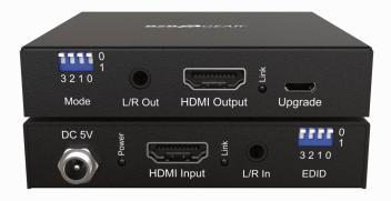
The BG-AEE is a HDMI 2.0 Audio Extractor and Embedder. It has two modes: audio extraction via L/R output from HDMI input source, and the other mode is for removing the original audio of HDMI source and embedding auxiliary audio via L/R input to the HDMI output. It also features EDID dip switches with the ability to lock the video signal to various formats to ensure signal quality.
