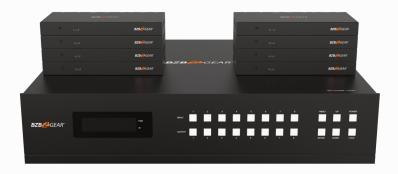
These 4K 4X4 (BG-UM44-100M-KIT) and 8X8 (BG-UM88-100M-KIT) HDMI HDBaseT matrix switches feature HDMI outputs mirrored to simultaneous HDBaseT outputs. The HDBaseT outputs can extend a 4K@60Hz 4:4:4 video signal at distances up to 328 feet (100 meters) over a single Cat5e/6/7 cable.
