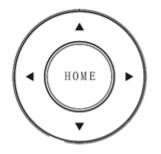
Move camera lens up ▲ Move camera lens down ▼ Move camera lens to the left ◄ Move camera lens to the right ► Return camera lens to center [HOME]
