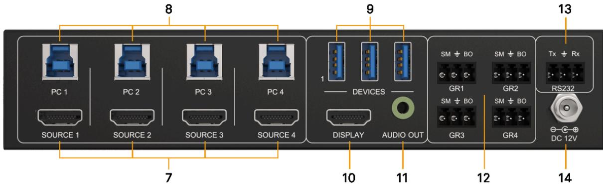
7. **HDMI SOURCE 1-4:** Connect up to 4 HDMI source devices (PC, MAC, etc.).
