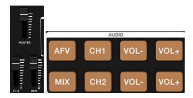
The BG-QuadFusion-JR supports analog balanced audio input and output, HDMI audio extraction, as well as audio matrixing using the Audio Follow Video (AFV) and MIX functions.
