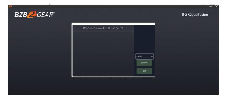
Upon opening the application, your device should be listed in the box in the center along with its IP address if both the device and computer are on the same network. You can also use the dropdown on the right to select a different internet adapter if your computer has more than one or to search again if the device was not found initially.
