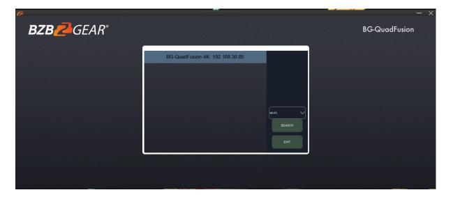
Double click on the device name in the center to access the virtual production switch.
