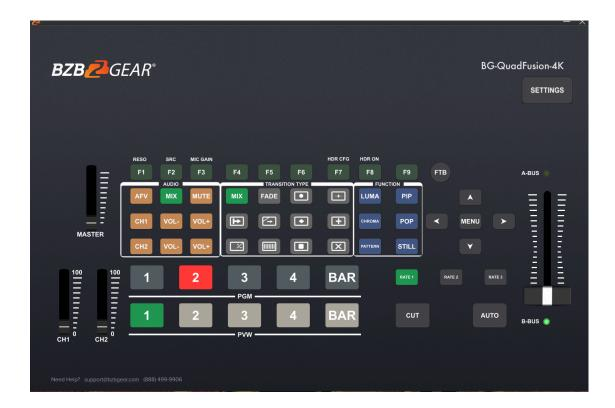
The virtual software functions exactly the same as if you were pressing the buttons on the unit itself and it will cause the physical unit to mirror your actions. NOTE: T-Bar and volume sliders will re-adjust when they are physically moved on the unit.
