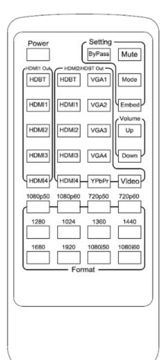
**HDMI1 Out**: Source selection for HDMI output 1 when in Matrix Switcher mode.
