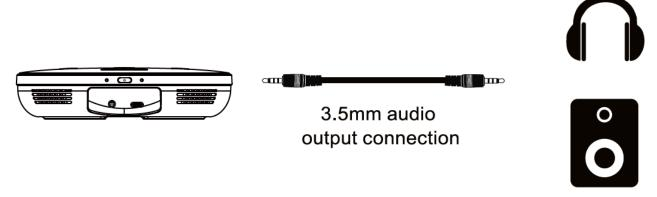
1. Connect the BG-OMNITALK to either headphones or an external audio system using a 3.5mm stereo audio cable.
