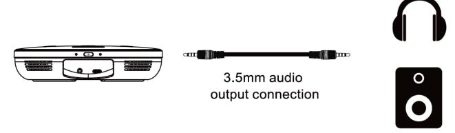
1. Connect the BG-OMNITALK-PRO to either headphones or an external audio system using a 3.5mm stereo audio cable.
