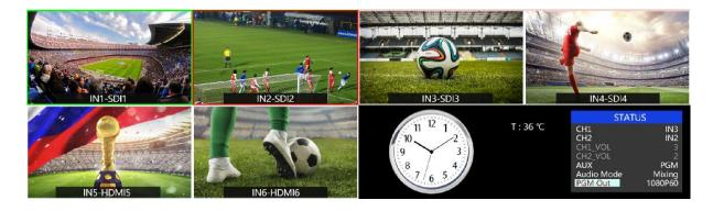
The lower right corner of the display features the menu and status information. The CH1, CH2 are the channel selection of the 2 audio sources for the audio mixer. There is a real-time Digital clock/Analog clock displayed beside the menu.
