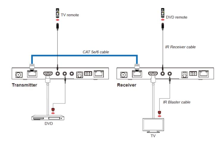
**Note:** When the angle between the IR receiver and the remote control is  $\pm$  45 °, the transmission distance is 0-5 meters.
