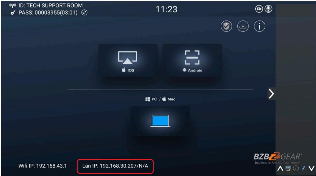
**Note:** When it shows “N/A” this means the Connexio is not connected to the LAN (Local Area Network) by CAT cable or it failed to get an available IP address from the router.
