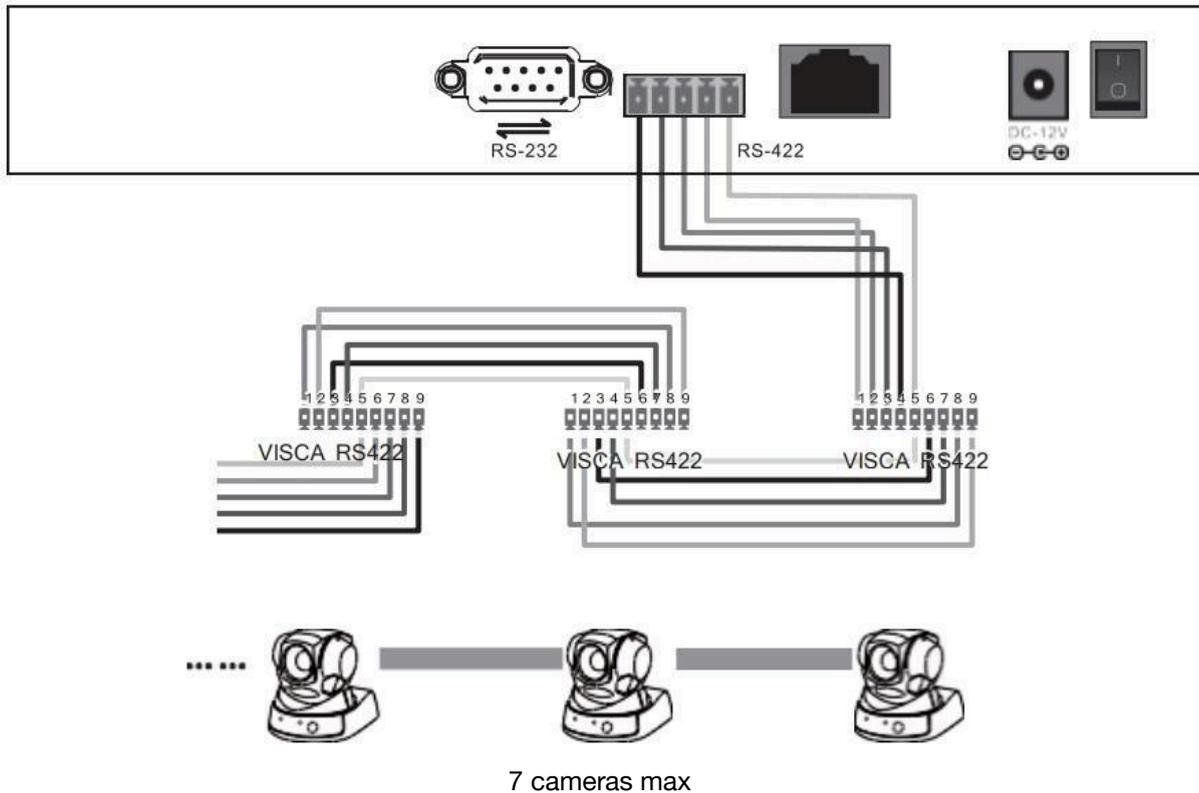
When using RS422 bus connection mode, the third pin (**Ra**) of the controller is connected to the **TXD IN-** of the camera, the fourth pin (**Rb**) of the controller is connected to the **TXD IN+** of the camera, the first pin (**Ta**) of the controller is connected to the **RXD IN-** of the camera, and the second pin (**Tb**) of the controller is connected to the **RXD IN+**
