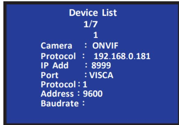
1. Press the **[SETUP/MENU]** button to enter the settings interface, move the joystick up and down to select option 3 Device List press the **[ENTER]** button to view the added devices.
