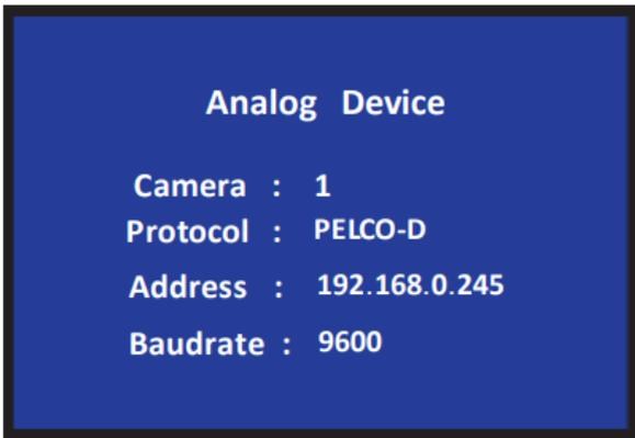
1. Long press the button on top of the joystick handle to switch the analog mode.
