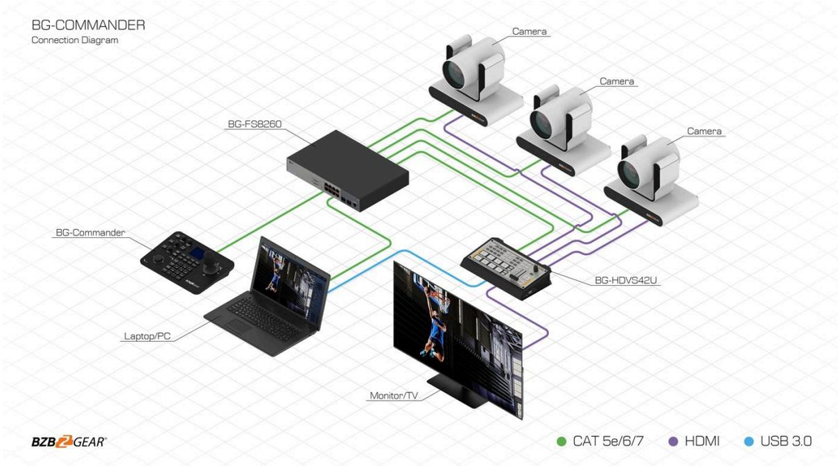
Camera and keyboard need to be connected to the LAN.
