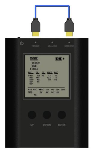
In this mode, BG-AVTPG-MINI offers a link quality estimator using a Character Error Detection mechanism to HDMI 2.0 specifications. The estimator can provide a basic link quality evaluation regarding the cable or any other HDMI link connected to BG-AVTPG-MINI.
