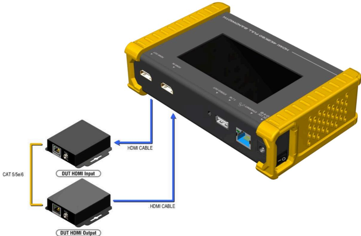
Procedure of Loop Test: \*only support 1080p@60, 4K2K 30Hz and 4K2K 60Hz resolutions
