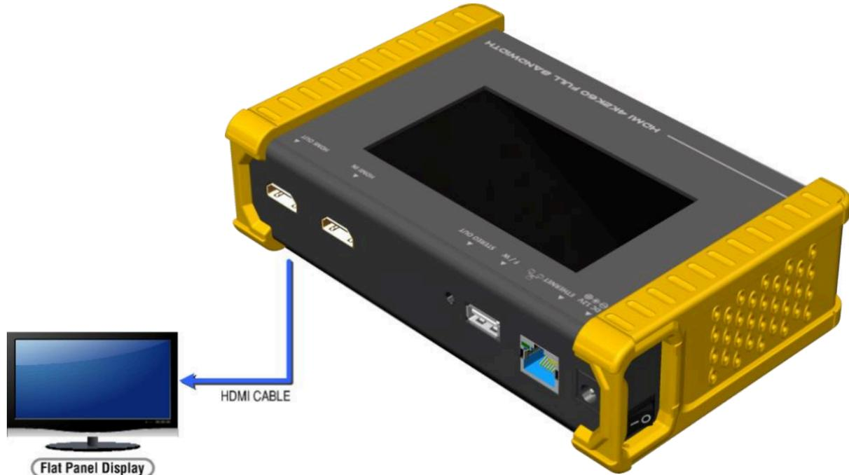
After making the physical connections between BG-AVTPG-4K and the display device. Users can select different generator functions to display on the sink device under test.
