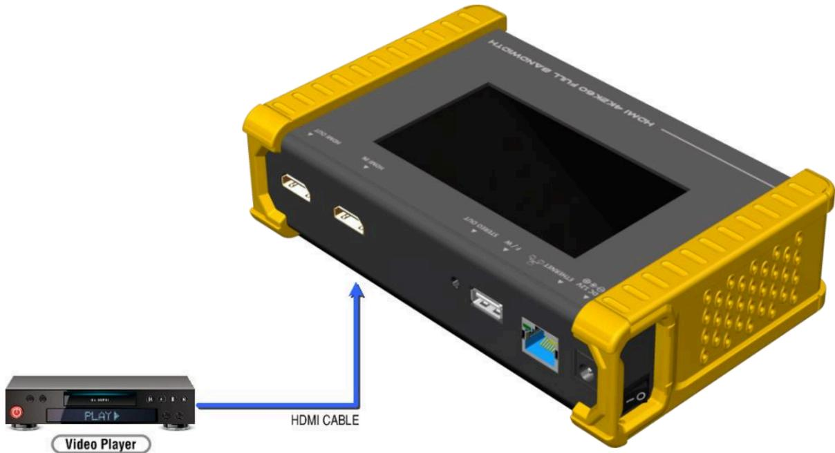
1. **Source Information from the HDMI source.** In the Test/Source menu, users can touch the read/refresh button to get the video format, source audio, and packet information from the HDMI source device.
