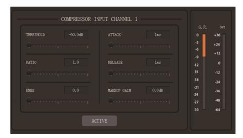
**THRESHOLD:** The level that the signal above it will be compressed, with a scale of [-60.0, 0.0]dB.
