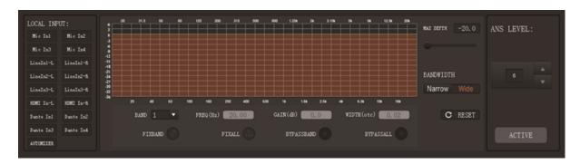
**MAX DEPTH:** The maximum amount of gain that the module allows to reduce, with a scale of [-20.0, 0.0] dB.
