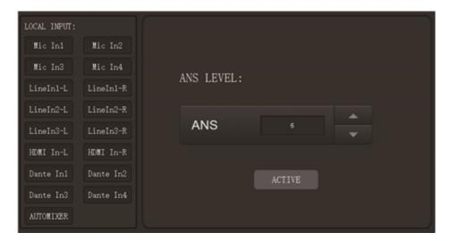
**LOCAL INPUT:** Shows source signals that are available to have access to the ANS process. AUTOMIXER refers to mixed signals after the AUTOMIXER process.
