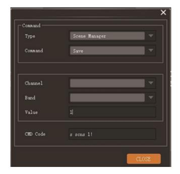
All RS-232 control commands, such as, Scene Management, I/O Control, Modules' Configuration, and Device Information, can be found in the page. The command code will be listed at the bottom of this page once you have selected the Type, Command, Channel, Band from the drop-down box and entered its value.
