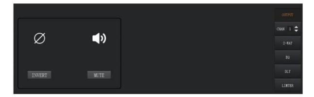
**INVERT:** When pressed, inverts the polarity of the signal on the channel.
