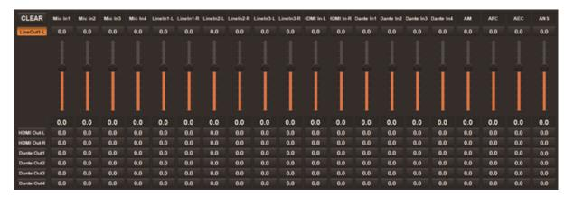
As shown above, the horizontal line stands for output channels and the vertical for input channels (AM, AFC, AEC and ANS exceptable).
