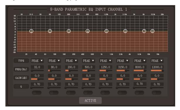
TYPE: Provides 3 types of band/filter, with High Pass, Low Pass and Peak optional.
