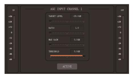
**TARGET LEVEL:** The desired output signal level, with a scale of [-20.0, 0.0] dB.
