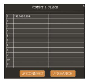
**Step 5:** Choose the audio processor's IP address and click CONNECT, then the processor will be connected with the host computer. After connection, the CONNECT & SETUP box (see the figure below) will pop out. You may close it directly if no such operation is needed.
