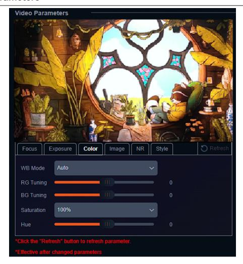
From the Video Parameters tab users have several options to manually control the image captured from the camera. Controls are broken into 6 sub sections: Focus, Exposure, Color, Image, NR, and Style. A preview image is shown above the settings so users can see their changes in real time.
