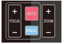
FOCUS + (near) : Press to adjust the lens focus.
