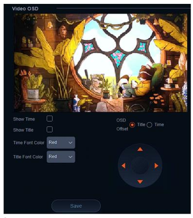
Video OSD or On Screen Display gives users the option to display the Device Name, Date, and Time, on the stream of the camera. This can be useful in easily identifying cameras when multiple are in use simultaneously in a production or security type setup.
