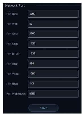
Network Port allows users to modify port settings for various camera streams. The port follows the IP address but before stream specific information when connecting to various stream types.
