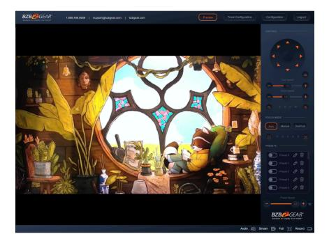
After successfully logging into the management interface, the web portal will enter the "Preview" tab. In Preview, users can control pan/tilt, zoom, focus, video capture, sound, focus, full screen preview, as well as set and recall preset positions and configure the "Home" preset position.
