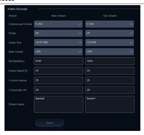
Covered by one or more claims of the HEVC patents listed at patentlist.accessadvance.com From the Video Encode tab users can edit the following parameters for the main and sub streams:
