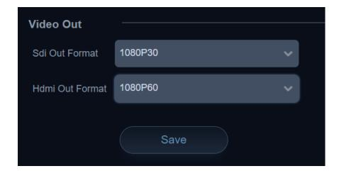
Video Out is used to adjust output resolution of the camera to its physical HDMI and SDI outputs.
