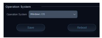
**Operation System** is used to control and limit the USB output resolution and refresh rate when connecting to Windows OS or MAC OS platforms to ensure the best possible performance.
