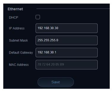
Ethernet settings allow users to change or modify how the camera is accessed on the network.
