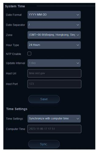
**System Time** allows users to edit date and hour formats, time zones, hour type (24hr/12hr), if an NTP server is used or if the camera syncs to the connected computer via the web interface.
