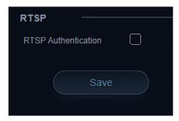
RTSP Authentication when enabled required users to enter the camera's login credentials directly into the RTSP stream URL to gain access as shown: rtsp://USER:PASS@{IP}:port/stream info.
