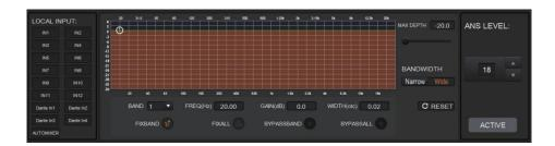
**MAX DEPTH:** The maximum amount of gain that the module can reduce, with a scale of [-20.0, 0.0] dB.
