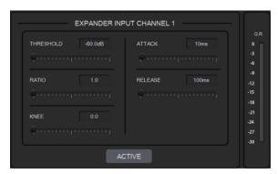
**THRESHOLD:** The level that the signal below it will be identified as noise and attenuated, with a range of [-60.0, 0.0] dB.
