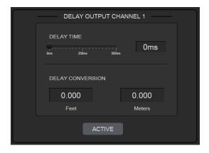
**DELAY TIME:** Adjusts the delay time of the output audio signal, measured in
