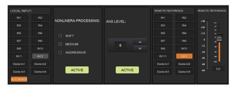
**LOCAL INPUT:** Shows source signals that are available to the AEC process. AUTOMIXER refers to mixed signals after the AUTOMIXER process.
