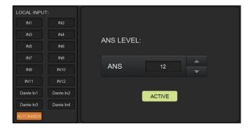
**LOCAL INPUT:** Shows source signals that are available to the ANS process. AUTOMIXER refers to mixed signals after the AUTOMIXER process.
