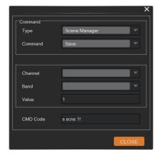
All RS-232 control commands, such as, Scene Management, I/O Control, Modules' Configuration, and Device Information, can be found in the page. The command code will be listed at the bottom of this page once you have selected the Type, Command, Channel, Band from the drop-down box and entered its value.
