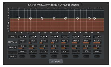
**TYPE:** Provides 3 types of band/filters: High Pass, Low Pass, and Peak.
