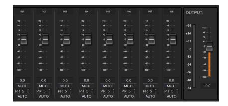
**FADER:** Each MIC input channel has a fader to adjust its signal level. It controls the mixed volume on the input channel.
