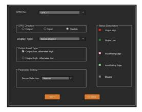
Users can configure the GPIO function as needed and see details on the GPIO Setting page. Users can also check the GPIO status via the GPIO LED at the top-right corner of the main page.
