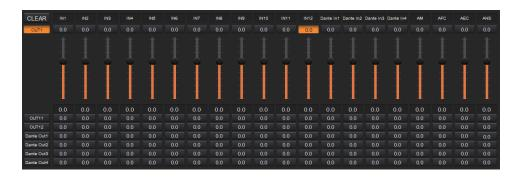
As shown above, the horizontal lines are output channels and the vertical are input channels (except AM, AFC, AEC and ANS).
