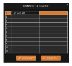
**Step 5**: Choose the audio processor's IP address and click CONNECT, then the processor will be connected with the host computer. After connection, the CONNECT & SETUP box (see the figure below) will pop up. You may close it if no such operation is needed.
