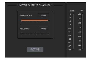
**THRESHOLD:** Shows signal levels above the threshold that will be attenuated, with a scale of [-60.0, 0.0] dB.
