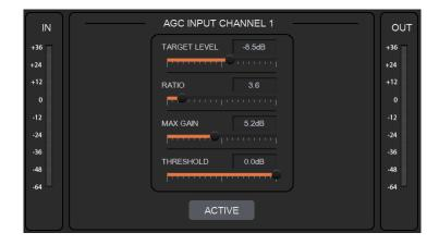
**TARGET LEVEL:** The desired output signal level, with a scale of [-20.0, 0.0] dB. **RATIO:** The compression ratio of signals above the target level, with a scale of [1.0, 20.0]. If the value sets to 2.0, it means that signals above that target level will be amplified twice
