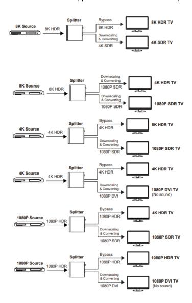
**Note:** If the source resolution is downscaled and converted to 1080P DVI according to the EDID of display devices, it will be output without sound on the TV.
