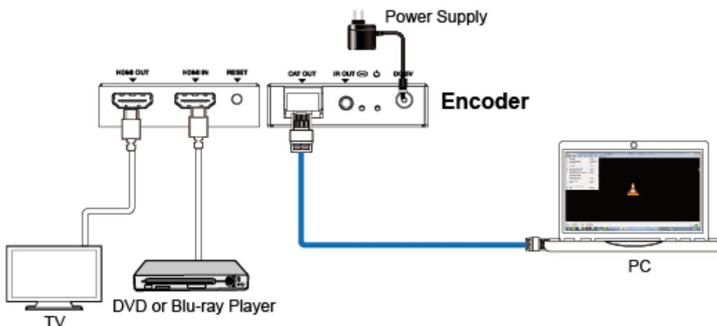
Figure 1: Video Stream connection diagram
