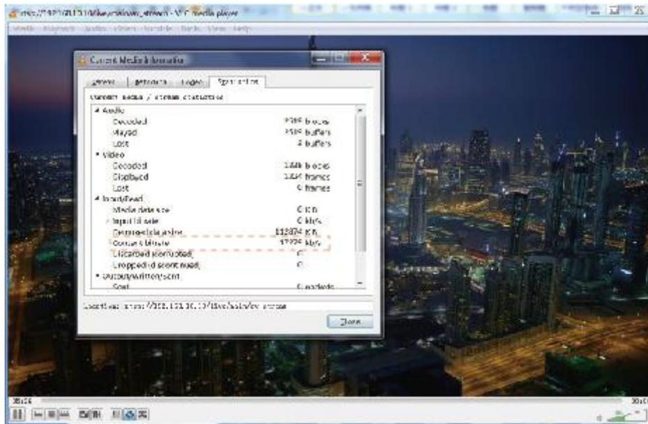
**Note:** The bitrate is floating up and down when you check it. This is a normal phenomenon.
