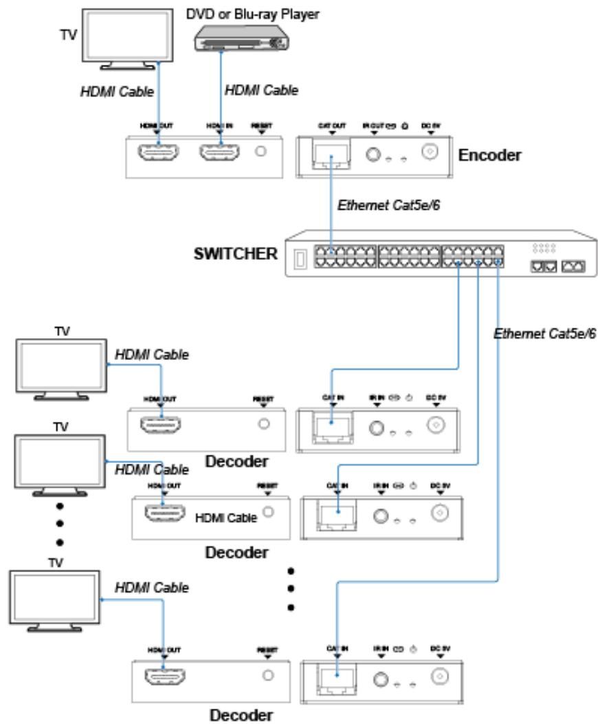
Figure 3: Encoder connects Decoder via switcher
