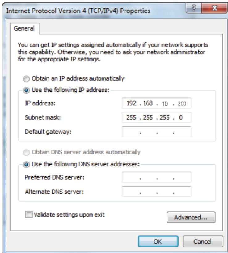
**Notice:** The IP address of the computer and Encoder should be in the same network segment. As the Encoder's IP address is 192.168.10.10, the computer's IP should be 192.168.10.X (X contains 1~255 except 10).
