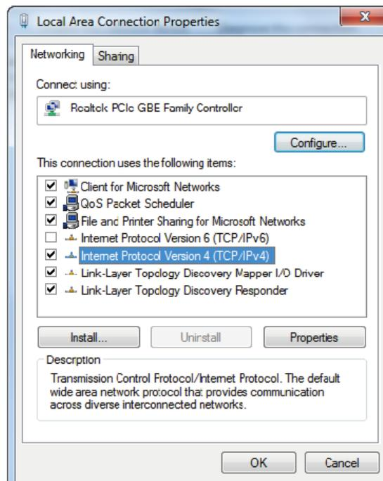
Choose "Use the following IP address" , input 192.168.10.200 as IP address, 255.255.255.0 as Subnet mask, and then click on OK, click on OK again.
